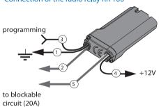
Wire 1 (Black) of the locking relay ('Ground') should be attached to the car body or to the reliable conductor connected to the body or any regular power user. This wire should connected first during the installation.
